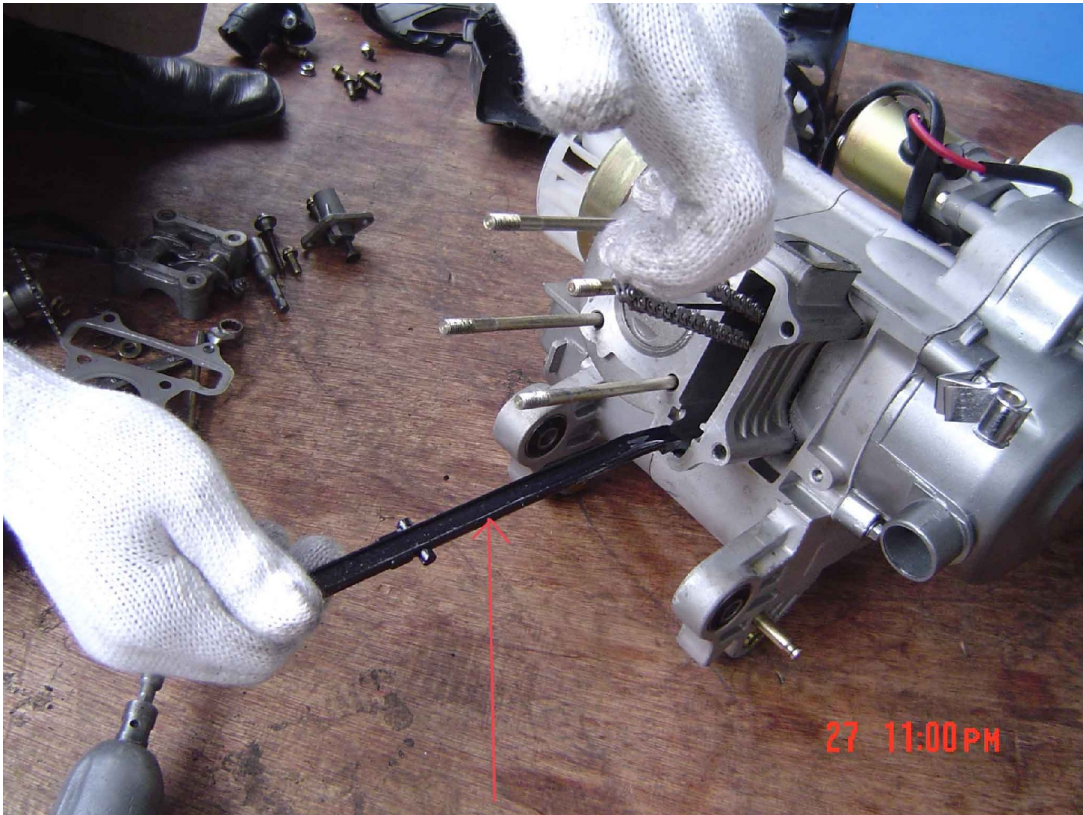
Fig. 13. Remove chain guide.
