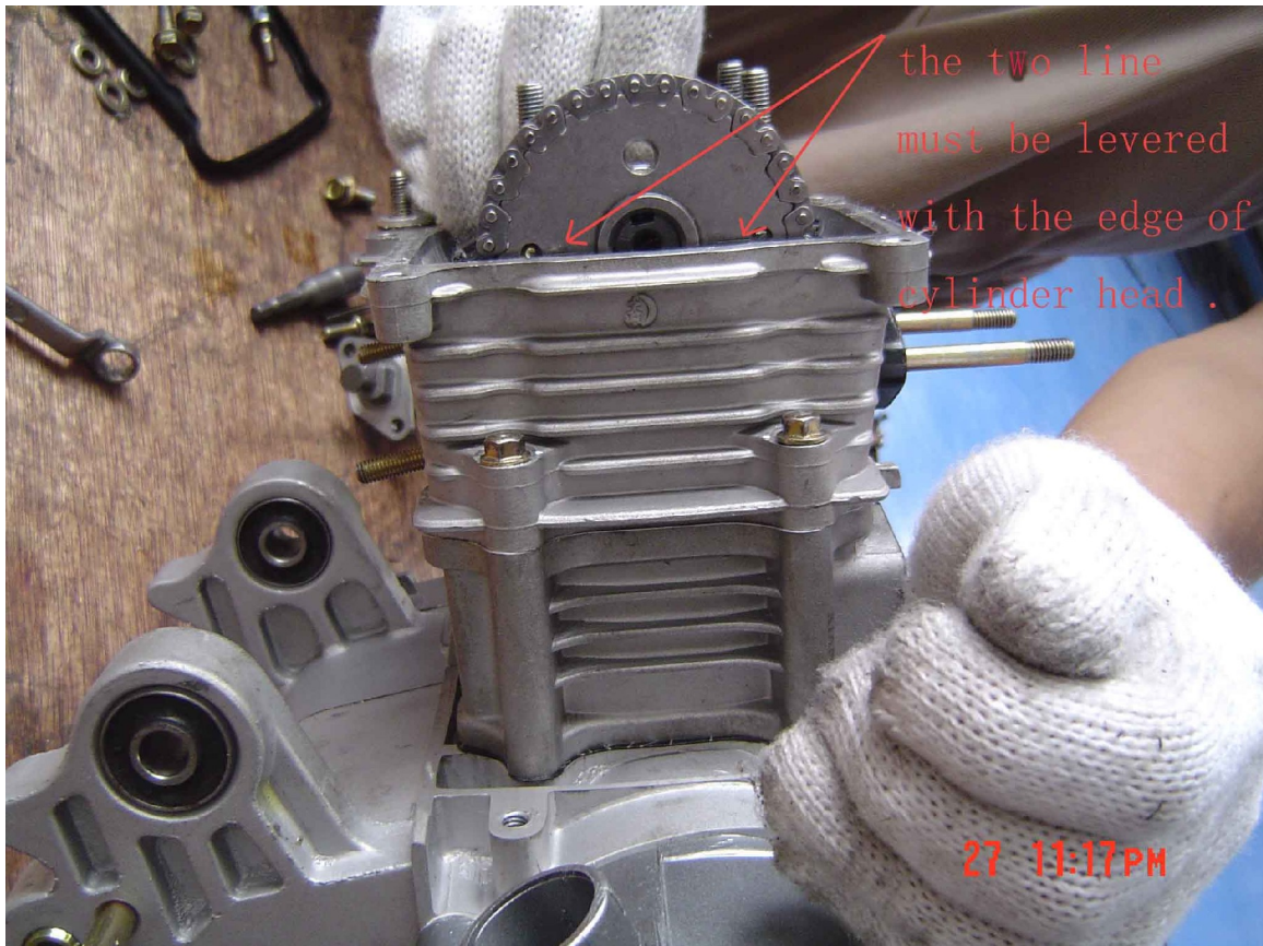
Fig. 9 a & b. Note the lines must be even with the edge of the head.
