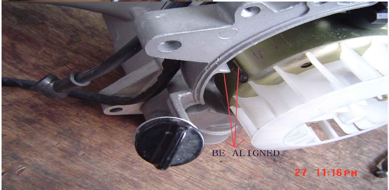
Fig 7. a & b. Install the cylinder head. Rotate the magneto and chain until the markings are lined up.
