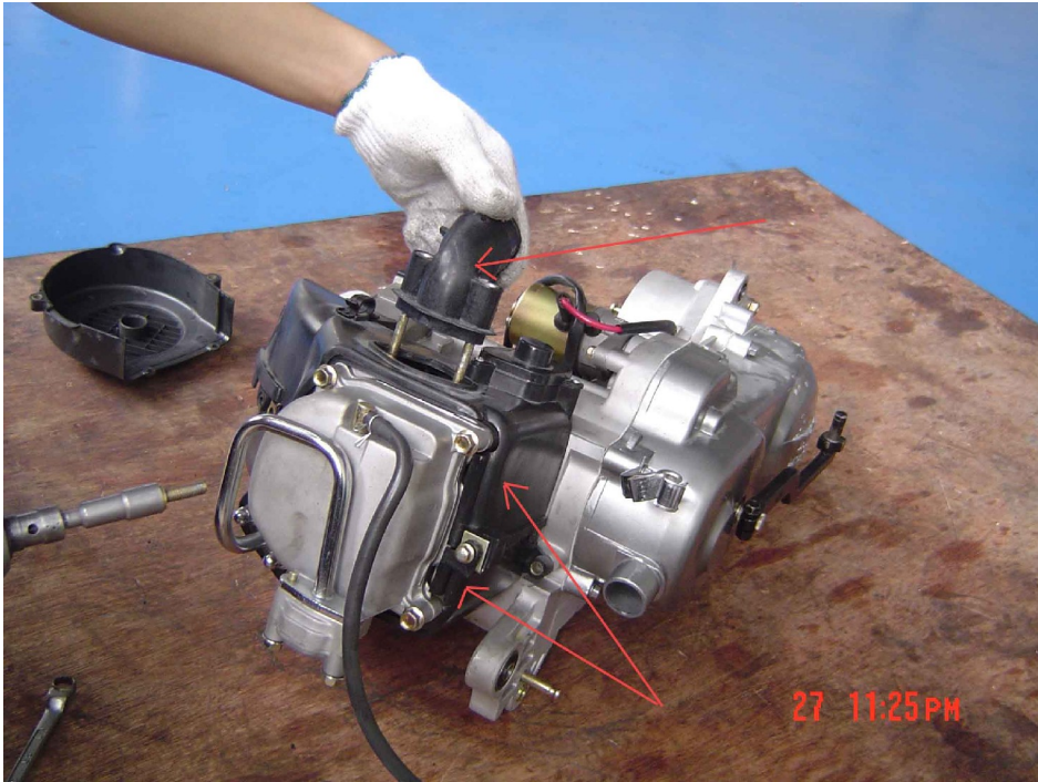
Fig. 16. Install carb inlet tube.
