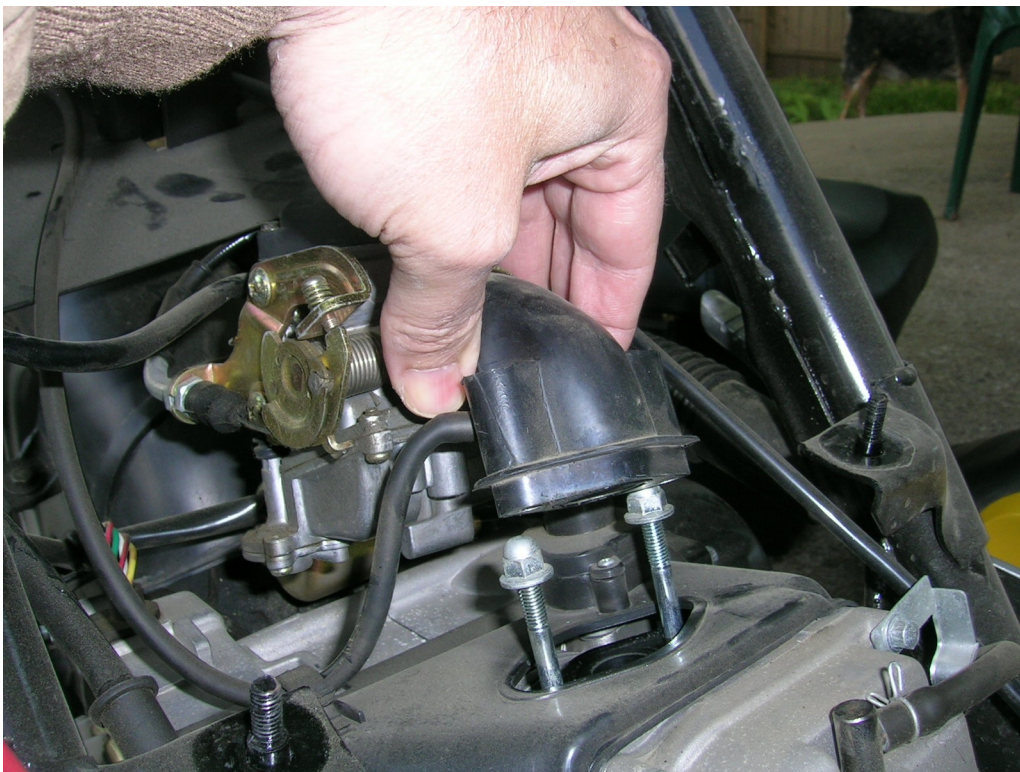
Fig. 3. Remove carb inlet tube.
