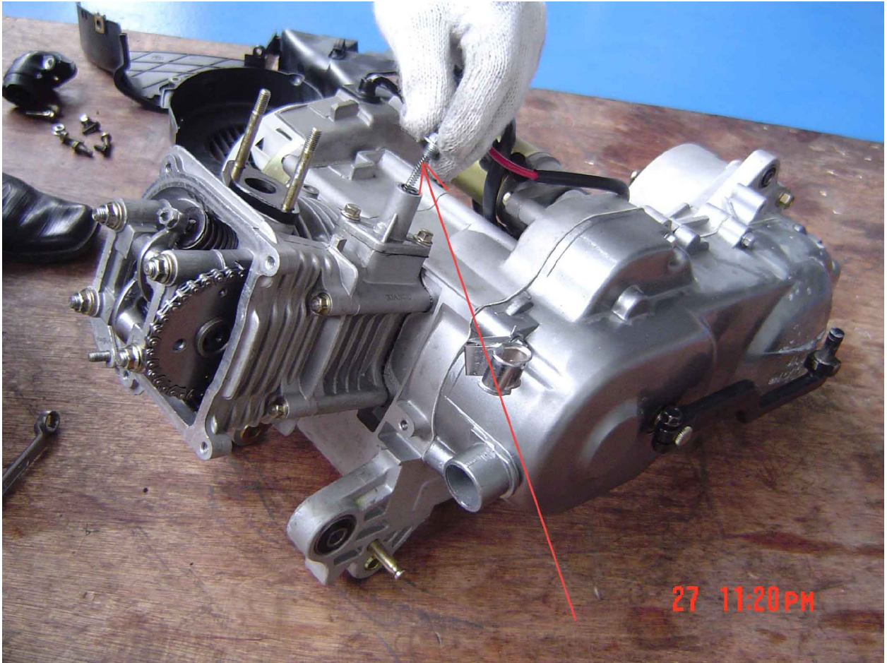
Fig. 12b. Install chain tension.
