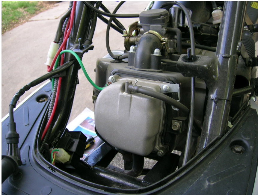
Fig 1. Body panels removed for full access to engine
