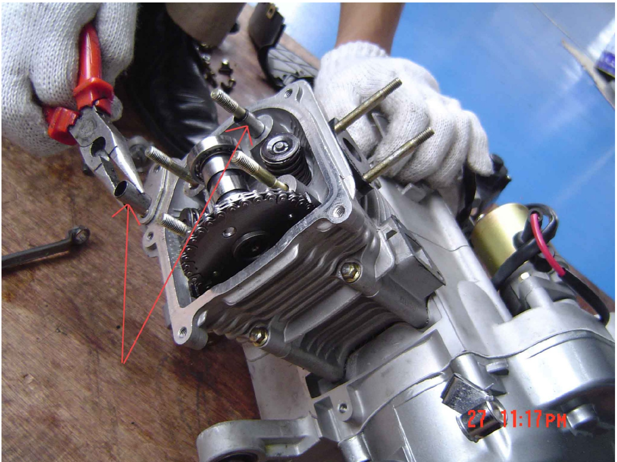
Fig. 10. Install alignment pins
