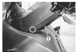
• Remove the handlebar front cover ②.
