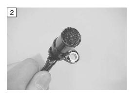
Check the speed sensor output voltage.
