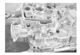
When installing the switch, apply SUZUKI BOND "1207B".
