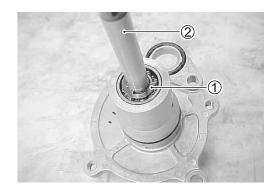
• Remove the mechanical seal using the special tool.
