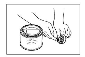
• First install the right wheel bearing, then install the left wheel bearing and spacer using the special tool.
