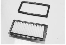
· Carefully use air hose to blow the dust from the cleaner element.
