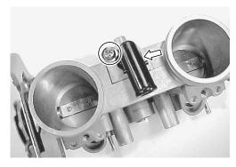
• Remove the throttle cable bracket.
