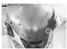
• Remove the wind screen brace 2.
