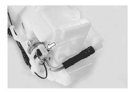
• Install the fuel level gauge.
