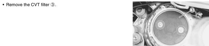
• Inspect the CVT filter for damage and dirt. If any defects are found, the CVT filter must be replaced.
