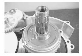
• Turn the primary slide pulley idle gear clockwise and open the primary pulley fully.
