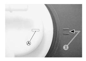
• Using the special tool, tighten the fuel pump ring locknut to the specified torque.
