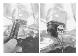
• Install the pulley position sensor ① with the sensor pushed toward the primary pulley shaft side.
