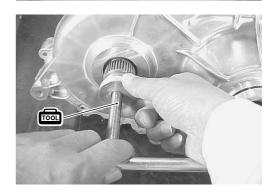
Apply THREAD LOCK SUPER "1360" to the primary pulley shaft bolt.
