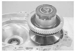
• Install the primary pulley shaft adaptor with the special tool.
