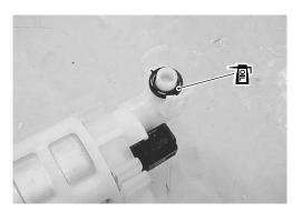
• Install the fuel pump to its holder and connect the lead wire coupler.
