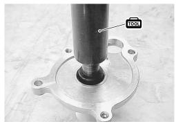
Apply a small quantity of the SUZUKI SUPER GREASE "A" to the oil seal lip.
