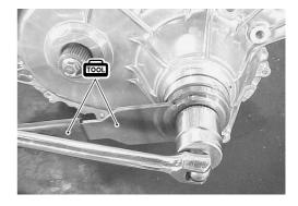
• Remove the secondary shaft adaptor with a bearing puller.
