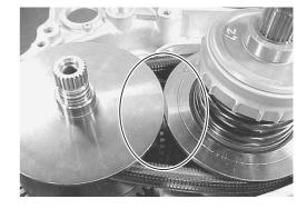
Check that the CVT belt is in parallel with the CVT cover mating face.
