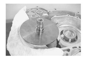
• Install the CVT belt so that the direction mark on the CVT belt points in the normal turning direction.
