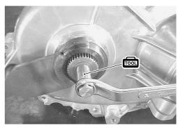
• Separate the CVT assembly by using 6 mm screws.
