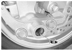
Apply SUZUKI SILICONE GREASE to the brake-lock shaft.
