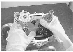
• Install the secondary pulley washer ③.
