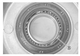
Apply SUZUKI BOND "1215" to the mating surface of the CVT casing.
