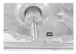
• Tighten the primary pulley shaft bolt to the specified torque with the special tools.
