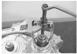
• Remove the primary pulley shaft bolt by holding the primary pulley shaft with the special tools.
