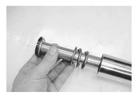
Apply THREAD LOCK "1342" to the cylinder bolt and tighten it to the specified torque.
