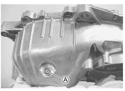
• Remove the primary pulley assembly.
