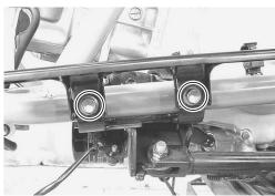
• Remove the engine from the frame.
