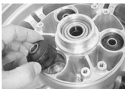
• Remove the dampers with the appropriate bar.
