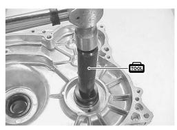
• Install the bearing retainer ①.
