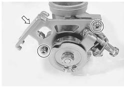
• Remove the synchronizing screws.
